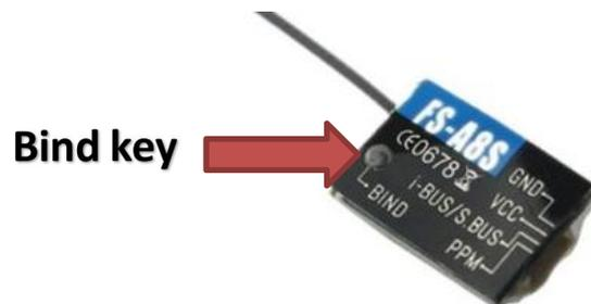
3. Exit the transmitter from the binding interface manually, and the status indicator of the receiver will be on.
